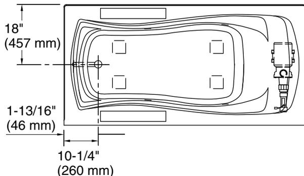
No change in measurements if connected with drain illustrated. (K-7166-AF)
