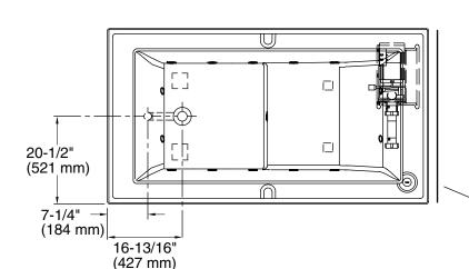
No change in measurements if connected with drain illustrated. (K-7193)
