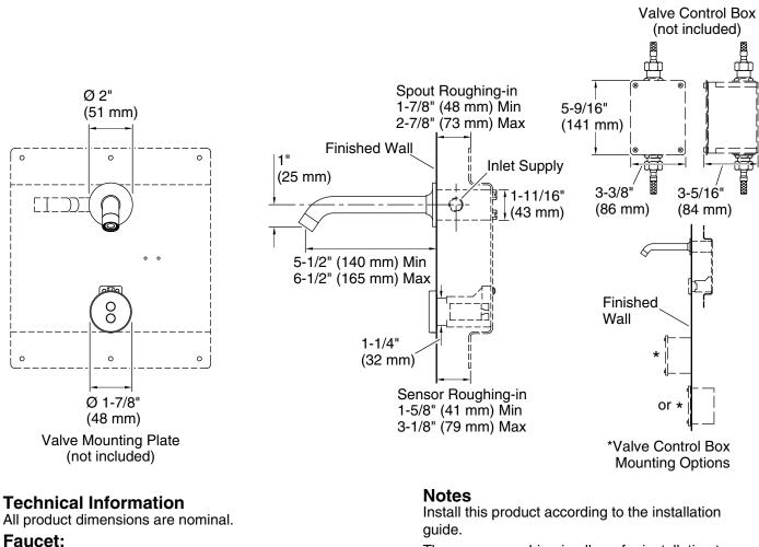
The sensor roughing-in allows for installation to a back splash or thicker finished wall than the spout roughing-in.
