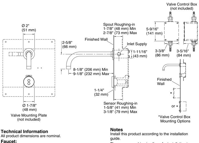
Flow rate:0.5 gal/min (1.9 l/min)Pressure:60 psi (4.1 bar)
