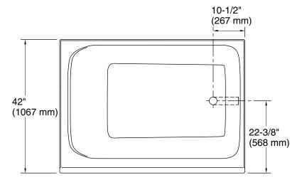
No change in measurements if connected with drain illustrated. (1381626)
