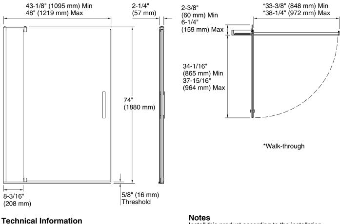
All product dimensions are nominal. Base-To-Wall 3/8" (10 mm) Radius – Max: Install this product according to the installation guide.
