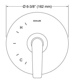
2-3/4" (70 mm) Thin Wall 3-1/2" (89 mm) Thick Wall If over 3-1/2" (89 mm) and up to 4-1/2" (114 mm). Use Deep Roughing-in Kit
