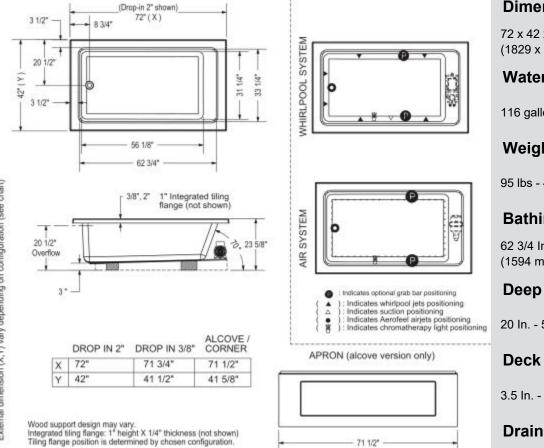
All dimensions are approximate. Structure measurement must be verified against the unit to ensure proper fit.
