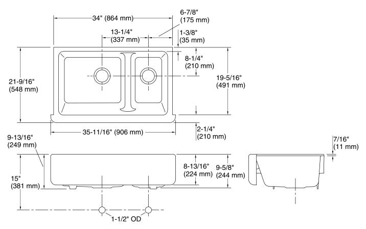
**Technical Information** All product dimensions are nominal. Bowl configuration: Off-set Large/small Min. base cabinet 36" (914 mm) width: Bowl area (Left): Length: 18-13/16" (478 mm) Width: 18-1/16" (459 mm) Bowl depth: 9" (229 mm) Water depth: 9" (229 mm) Length: 10-5/16" (262 mm) Bowl area (Right): Width: 18-1/16" (459 mm) Bowl depth: 9" (229 mm) Water depth: 9" (229 mm) Drain hole: 3-5/8" (92 mm)
