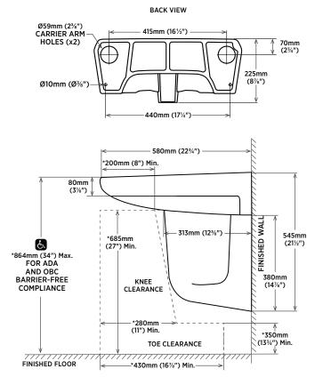
NOTE: \* Starred measurements comply with ADA and OBC barrier free accessibility requirements
