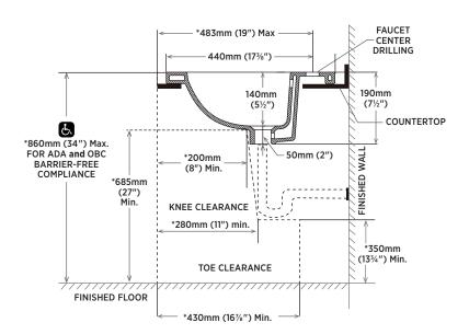
**NOTE:** \*Starred measurements comply with ADA and OBC barrier free accessibility requirements.
