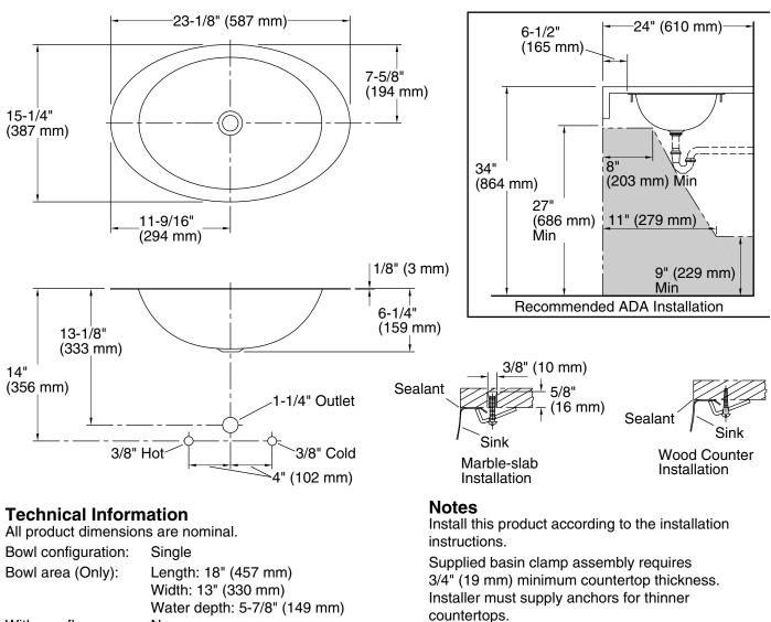
Water depth: 5-7/8" (149 mm)With overflow:NoDrain hole:1-5/8" (41 mm)Template:1000258-7, required, included
