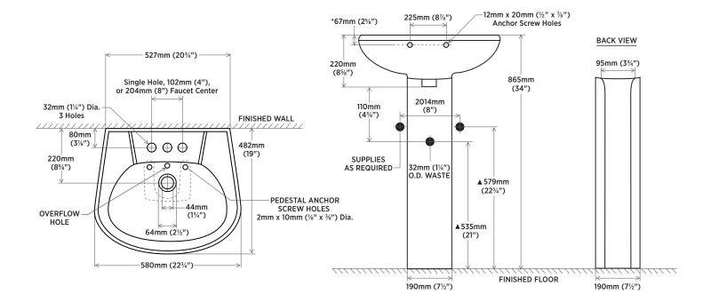
▲ NOTE: Dimensions shown for location of supplied and waste are suggested. Actual dimensions must be taken from fixture.
