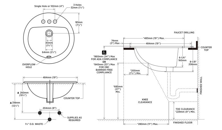
▲ NOTE: Starred measurements comply with ADA and OBC barrier free accessibility requirements. Dimensions shown for location of supplied and waste are suggested.
